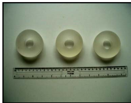
Figure 2. A photograph of the AEP60 polymer rings used in the development of the water content sensor
